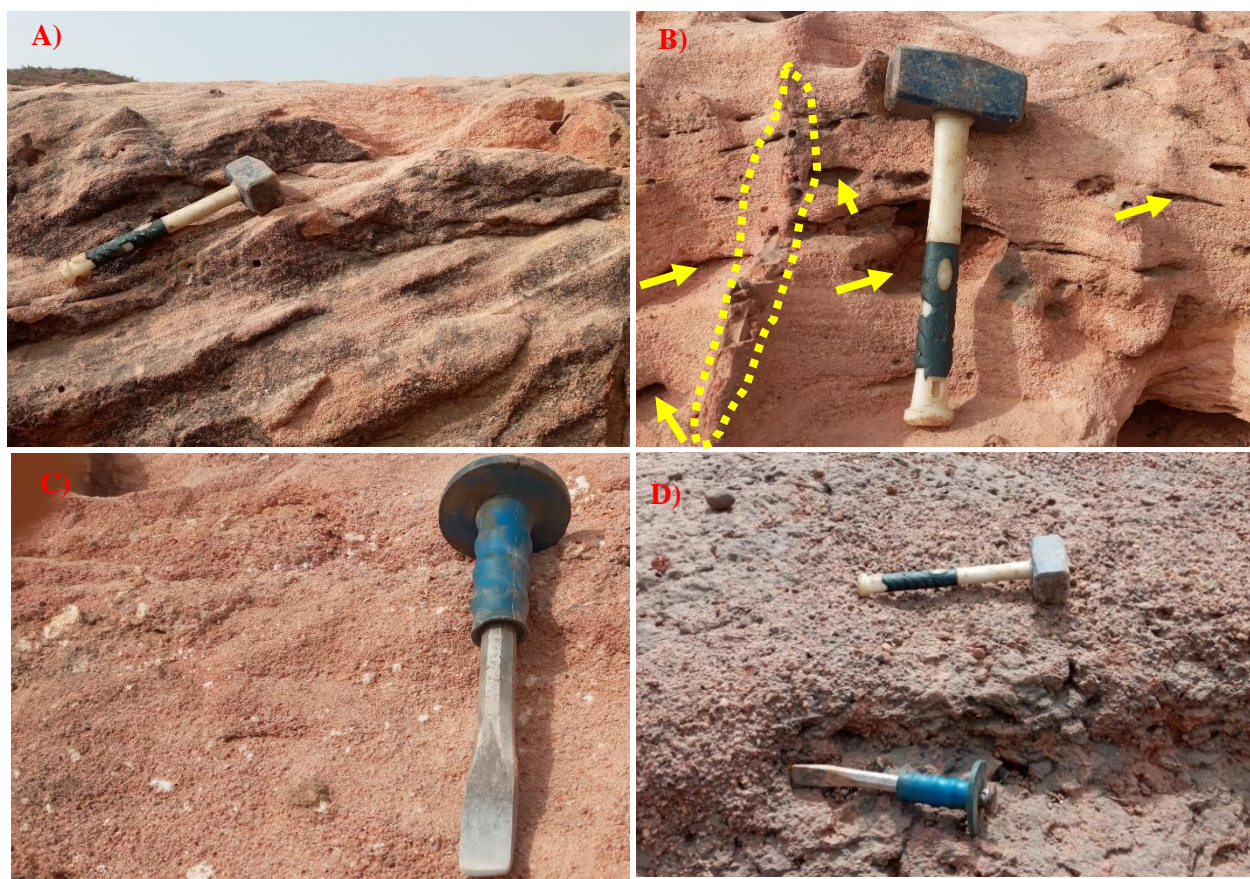
Figure 7 Field photograph of the sandstones of Bida Formation outcropping at Doko village. (a.) Medium grained sandstones with mega cross bedding structure, (b.) Brownish bioturbated (Yellow dotted circle and thick arrow) coarse grained sandstones, (c.) Brownish very coarse-grained sandstones with clay pod, (d) Ferruginized conglomeratic sandstones
