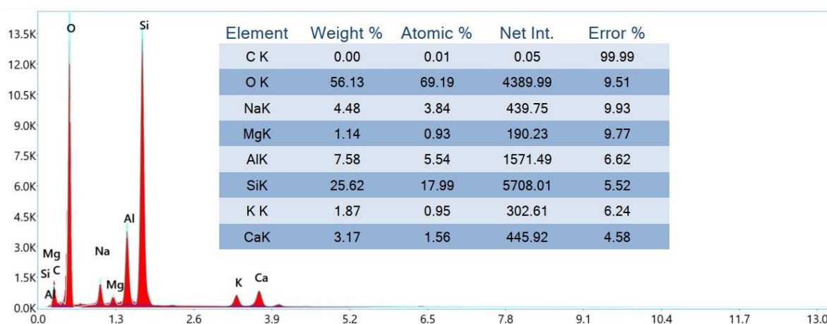
Figure 12 b Energy Dispersive Spectroscopy view of powdered eggshell adsorbent at spot B
