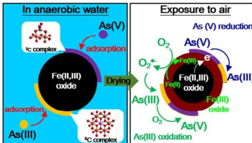
Figure 7a Mechanism of arsenic species adsorption in the environment (water and air; Source Liu et al., 2015)
