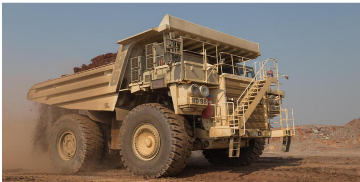
Fig 3: White Hybrid Diesel/Electric Hitachi Dump Truck used to cut Greenhouse Gas Emissions (Moore, 2014)
