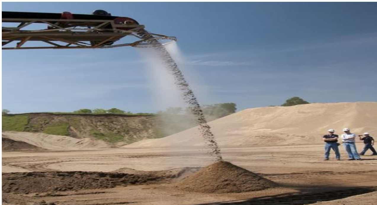
Fig 5. Dust Suppression: A Misting Ring Encloses the Material Stream in a Curtain of Atomized Dust (ECWeigh, 2023)
