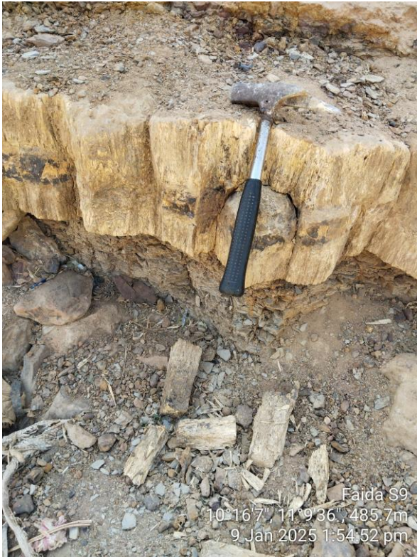
Plate 6: Sample S9 - Limestone, hard crystalline
