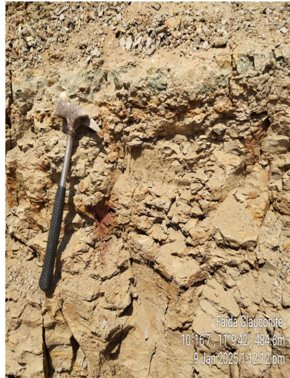
Plate 4: Sample S4 limestone enriched with glauconit
