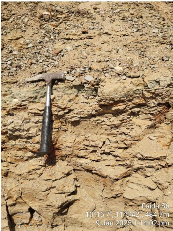
Plate 5: Sample S6 Light grey shale, fissile, laminated, disintegrated
