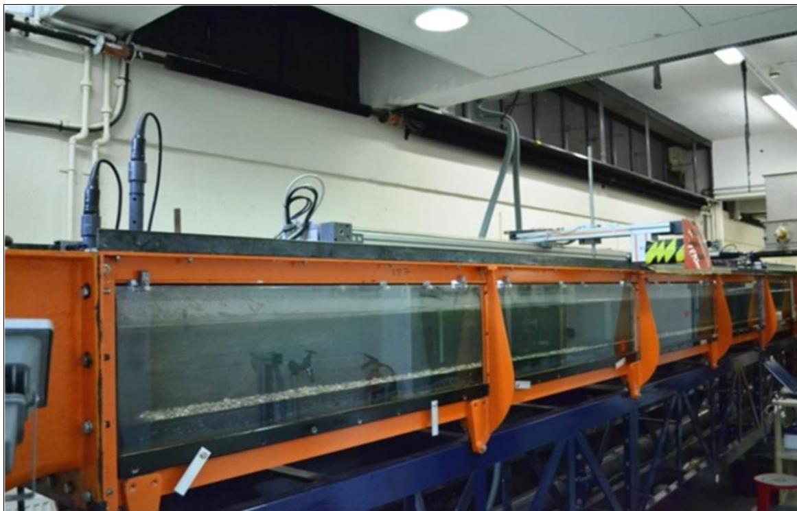
Figure 1b; Photograph of the open channel recirculating laboratory flume tank used in this research.
