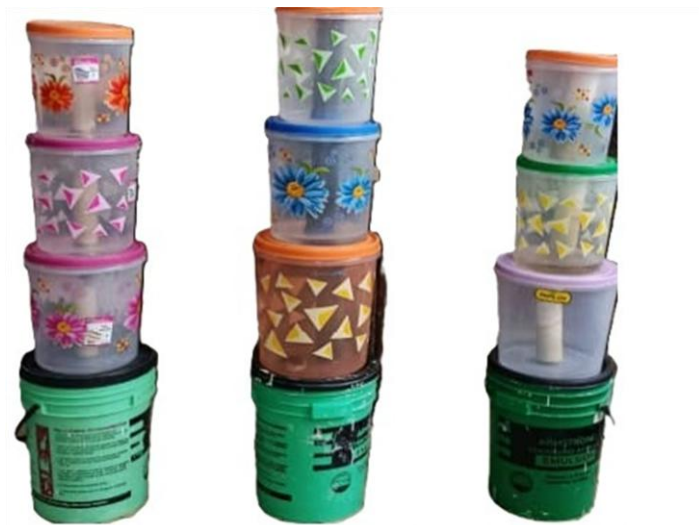
Figure 6b: Laboratory Set-up for Activated Carbon Filtration Unit
