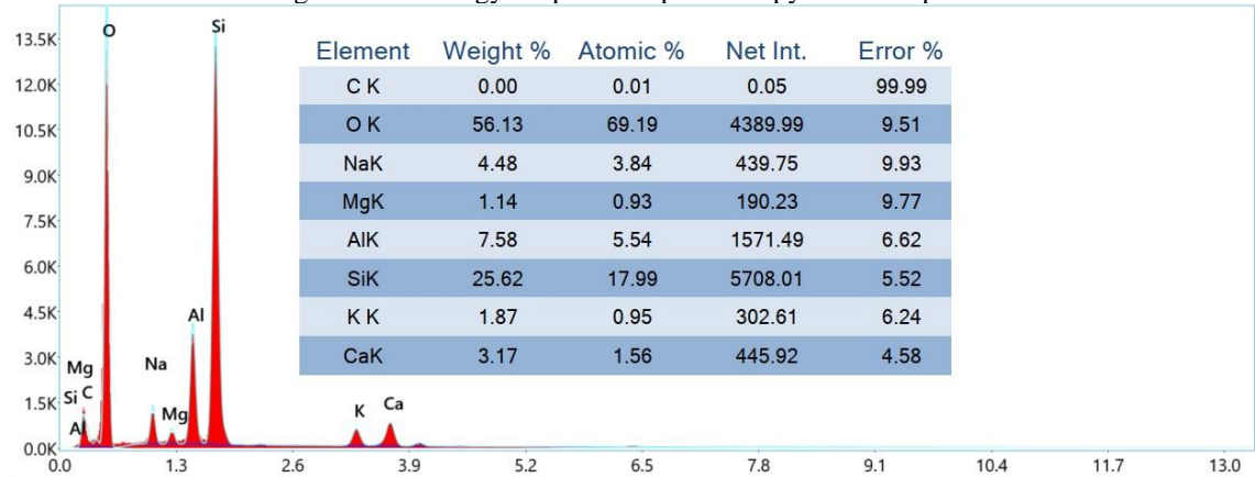
Figure 11aii: Energy Dispersive Spectroscopy results of Spot 2
