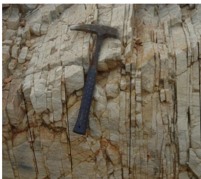
Plate 14. Vertical (parallel) joints on quartzite
