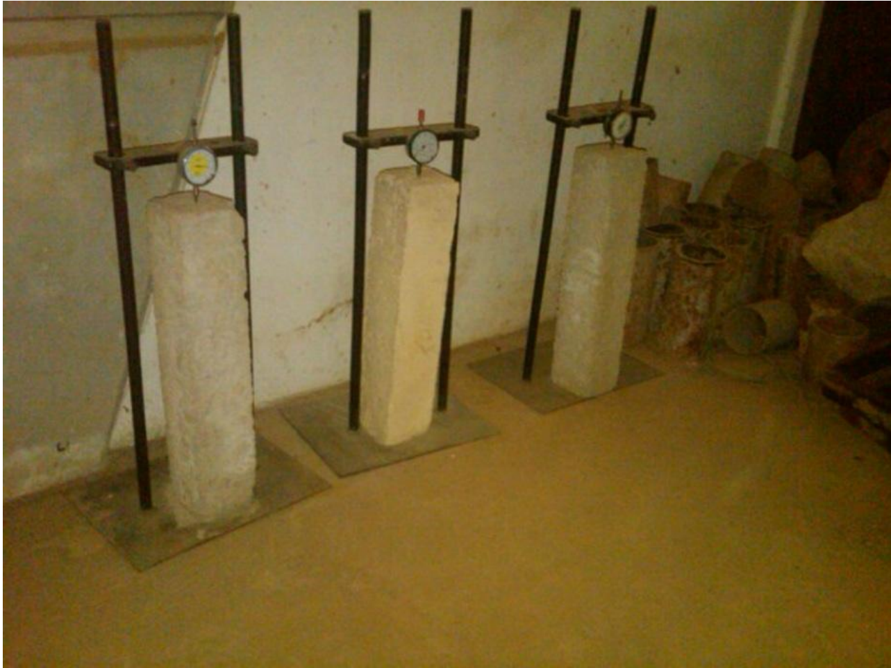
Plate 1: Laboratory setup of shrinkage deformation measurement
