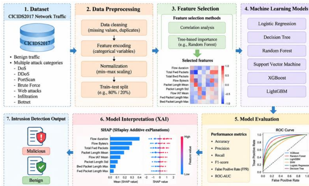
Figure 1. Overall workflow of the developed explainable artificial intelligence-based intrusion detection framework using network traffic analysis.
